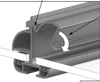
Roll the body of the capping around until the bottom edge of the capping touches the glass.
