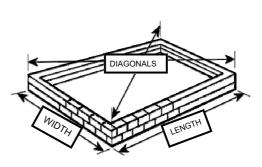
When building any base make sure the diagonal measurements are equal and everything is level.
