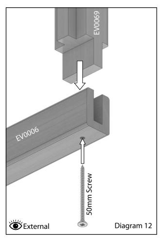
With the parts flat on the ground drill the pilot holes through each mortise in the cills and as before through the lap joint on the gable bars. Also drill pilot holes through the mortise holes on the gable bars ready for the door header. Fix the front cill to the gable glazing bar using a 50mm screw.
