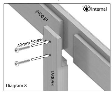
Now fit the right hand corner bar. Drill 2 pilot holes in the bottom of the bar (diagram 10). See diagram 4 for the position of these holes.
