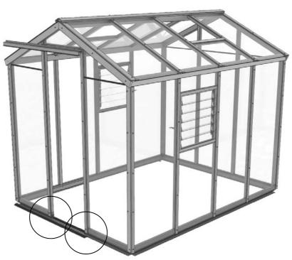
Now install the bottom door guide, start by fitting the door cill, diagram 35. Attach the cill to the base sections using the small plate (HE512M) and two 10mm nuts and bolts. (Keep this bracket as close to the ground as possible so it doesn't interfere with the threshold strip).
