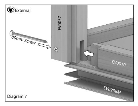
Once you have fixed the joint with the 80mm screw (diagram 7) fix the rear cill to the aluminium base with 25mm screws.
