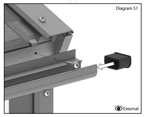
Start installing your gutter by inserting the stop end in one end. It is a good idea to secure this with a clear silicone. With help or the aid of a prop take gutter to greenhouse and fix the end with the stop end in, using a 25mm screw. This should be installed as high as possible on the side of the greenhouse to allow for a good fall when fixing the other end (diagram 51).
