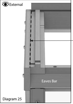
Glaze the remaining side sections as before. When you come to the front end glaze this as you did the rear end but when you install the roof corner cloaking strips leave out the last screw on the bottom left hand corner (marked with an 'X') as this will get in the way of the vertical door track support.
