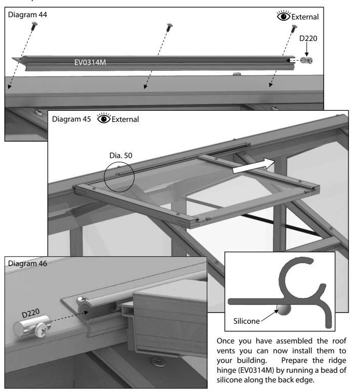
Then position this spaced equally over the opening in the roof. If you have the aluminium ridge cover then use the 13mm self taping screws, if it is the cedar ridge cover just use the standard 19mm screws. Secure one of the vent stops (D220) at one end of the ridge hinge channel.
