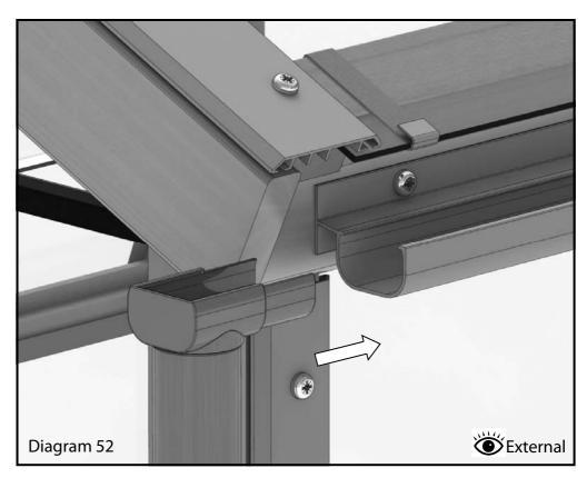
It is a good idea to support the downpipe once you have fitted it to the outlet as it is likely to drop off before you fit the downpipe bracket.
