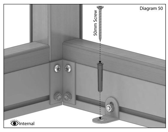
When you are happy with the final position of your greenhouse and all the sides are vertical and square you can fix the greenhouse to the ground. Use brown rawl plugs and 50mm screws to secure it through the base brackets previously attached (diagram 50).
