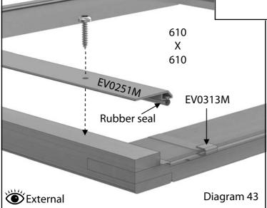
place with the vent capping (either cedar or aluminium) using the 25mm screws, diagram 43. Remember if you are using the aluminium capping system you will need to insert the rubber seal before fixing it in place.
