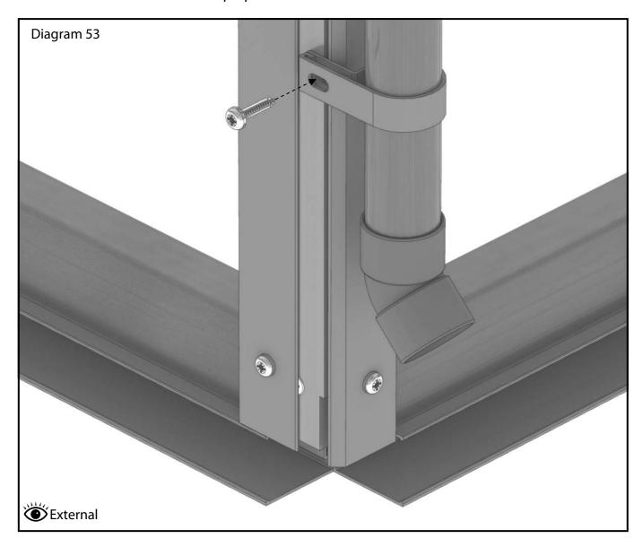
The downpipe bracket can be fitted at any point up and down the side corner bar to suite your application, use a 25mm screw to fix this. Attach the 45 degree bend at the bottom of the downpipe to direct the water away from the greenhouse.
