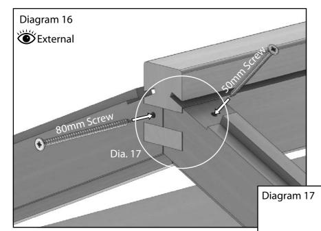
With help locate the ridge with the roof corner bars at both ends. Once into position, drill 2 pilot holes into each end as in diagram 16. Try to keep the angle something close to diagram 17, through the top face of the roof corner bars. This is to prevent the end or the screw coming through the bottom of the roof glazing bar. This angle will also give a much better and stronger fixing.
