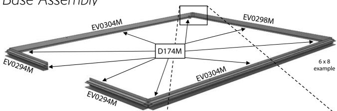
Lay out your aluminium base sections as the diagram shows. The base brackets should always be positioned either side of the door, in the corners, in the middle of the rear and equally spaced down the sides, as the diagram above shows. Use the crop headed bolts to fix these in place. The joining brackets fit in each corner to join the sections, these are fixed with standard bolts. The top holes will take a 25mm screw when the side cills are fixed to it.
