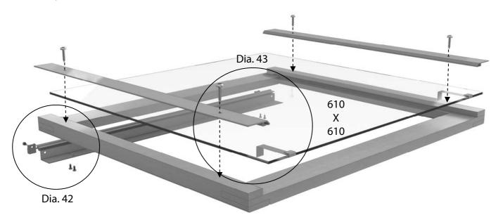
Take the vent frame that is ready assembled and fix the vent hinge to one end through the 4 pre drilled holes using the 19mm screws, diagram 42. Once this is in place fix the plastic vent filler (EV0323) also with a 19mm screw, its is **important** to make a pilot hole before fixing the plastic filler to prevent splitting.
