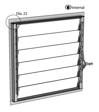
Now you have assembled the side trim the rubber seal flush with the ends. Attach the top and bottom of the louvre with the 12mm assembly screws. In each end. This locates with a screw channel in the side sections. Makes sure you pinch the glass retainers as this helps secure the glass when in place. You will find your louvre glass in the box with the louvre. You can install this now but it is easier to do so when the louvre is in the frame of the greenhouse.
