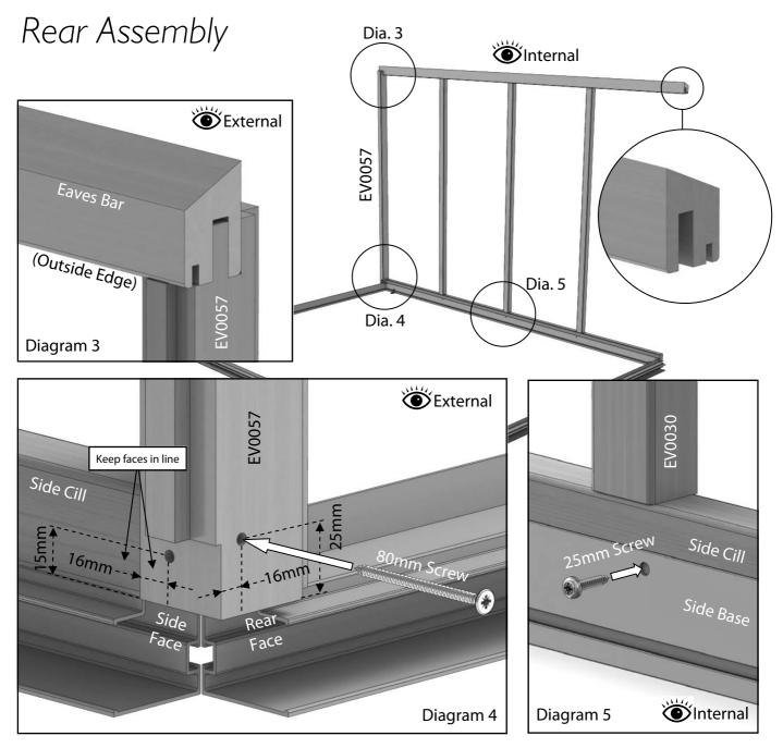
To install this section you will need a helper to hold the side in position or strap it to a set of steps. Drill two pilot holes in the bottom of the side corner bar as in diagram 4. The height of these holes should be about 15mm on the side face and 25mm on the rear face measured from the end of the bar, try to keep these at different heights to each other so the screws don't intersect each other.
