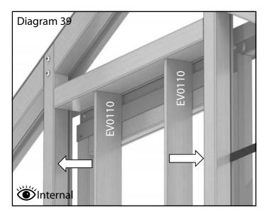
Standing on the inside of the greenhouse, with the door in the closed position you can install the door frame sides (diagram 39). Secure these with four 40mm screws per side. These should be fitted as close to the door as possible while still allowing it to pass by freely.
