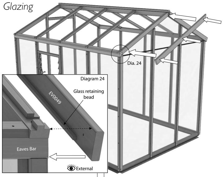
Install the rear glass in the same method as the side glass, the only difference is you have to stack the shaped panes on top using the glass separators. Make sure you have all the glass to hand when you are glazing this section. It is also a good idea to have an extra pair of hands to hold glass in place while you get the next section of glass in place. Always keep the glazing capping flush to the aluminium base level with the bottom of the glass.
