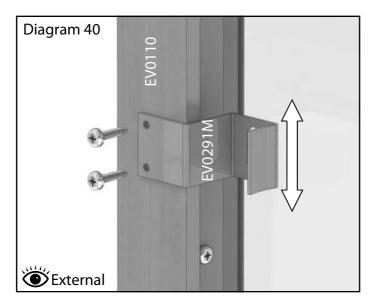
Once the door frame sides are installed you can fit the hasp and staple. First of all fit the hasp (EV0291M) to the right hand door frame side (diagram 40). Choose a position that best suites your reach, keep it clear of the handle fixings as this may prevent it from closing correctly. Fix this with two 25mm screws.
