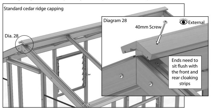
For the cedar cap fix one side in place then run a bead of silicone the full length of the cap where the next piece will join. Fix the second piece tightly against the first. Use 40mm screws for this cap.
