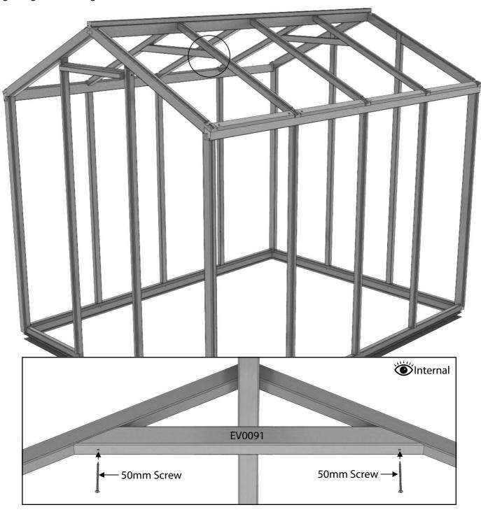
If your building is 12ft long you will be supplied with 2 ridge braces, fix these equally spaced in the building with 50mm screws.
