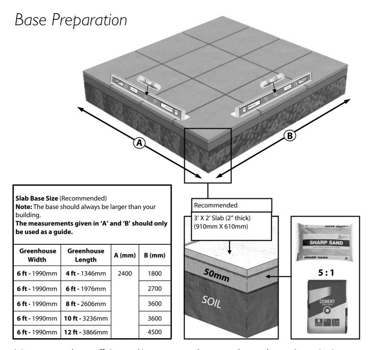
It is necessary to leave sufficient working room around your greenhouse when you're putting it up and also to allow for the possible need to replace a piece of glass in the future. If possible try and leave a space of 2ft/610mm around the greenhouse.
