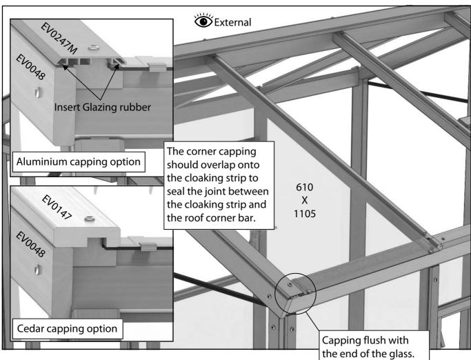
**Note**: Use countersunk screws where a vent is to be used so as the head of the screw doesn't prevent the vent from closing properly.
