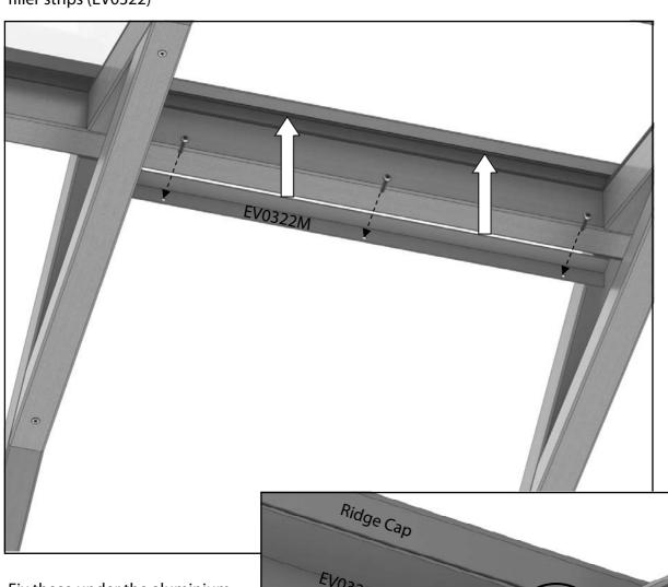
Fix these under the aluminium ridge cap with three 25mm screws. When in place silicone the two ends to seal any remaining gaps.
