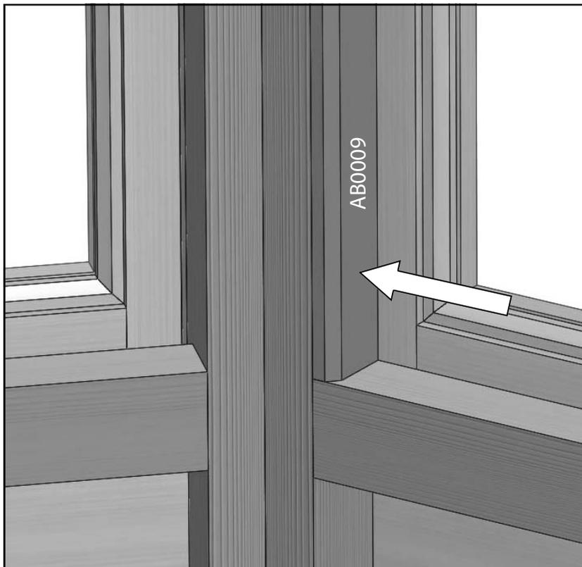
As with the architrave the window trims are fitted with four panel pins per side. (diagram 73). These need to be fitted to all window sections.
