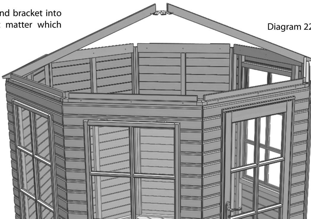
Then slot the rest of the roof bars into position. Fix them to the ridge bracket with 50mm screws as you go.
