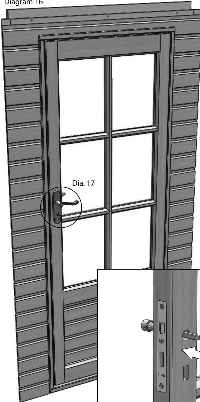
Before you can install the door section you need to fit the door handle. Slide the spindle through the lock to give you the position of the handle on the door. Fix the handle with the 3.5 x 25mm countersunk screws supplied.
