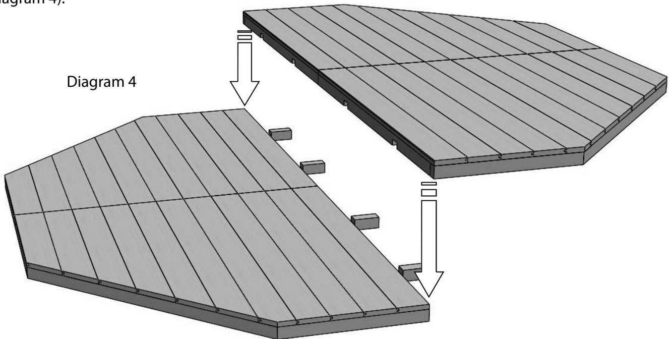
Check that the edges of the floor are in line before drilling pilot holes and fixing with 60mm passivated screws (diagram 5). Its is crucial to get the floor flat and level as this will affect how your building goes together and how well your windows and door will operate.
