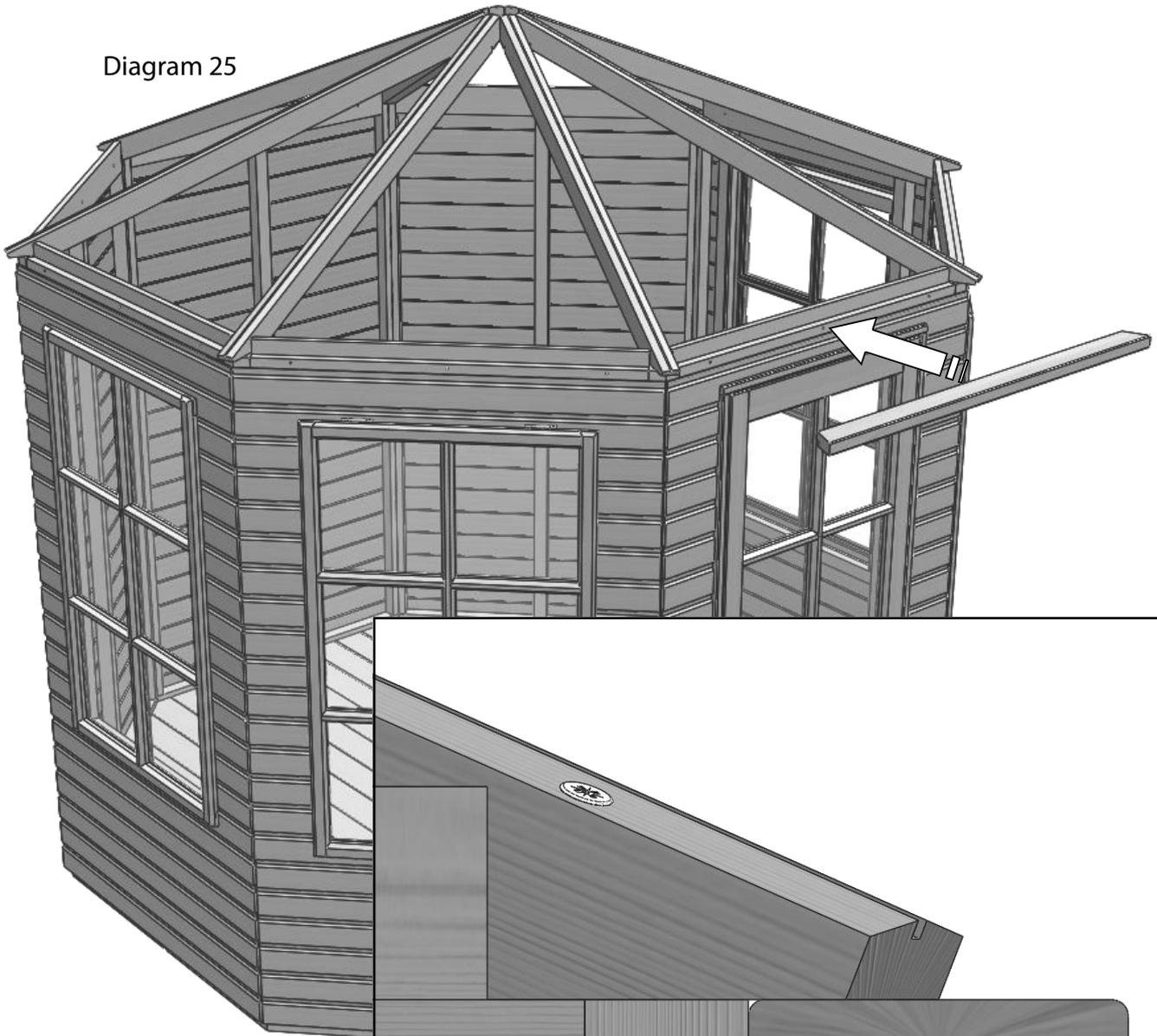
These are fixed to the top of the side panels (diagram 26). Push the soffits tight up against the underside of the roof bars. Screw position shown in diagram 27 overleaf.
