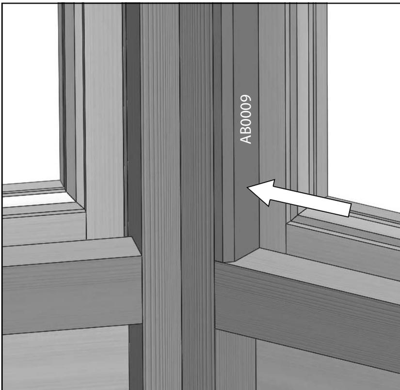
As with the architrave the window trims are fitted with four panel pins per side. (diagram 73). These need to be fitted to all window sections.
