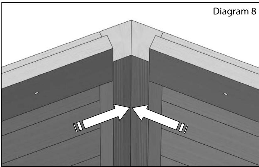
When fixing the panels bear in mind which faces will be most visible when you walk into the building. Try to keep the screw heads on the least visible faces where possible.
