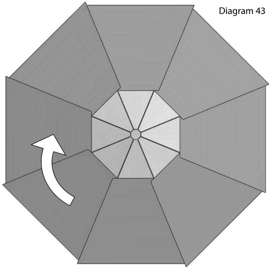
Now fit the smaller felt sections above the large ones. The bottom edge of the small sheet should be around 100mm below the top of the larger sheet to give a good overlap. In this position all the edges of both sheets should line up. Fix this as shown in diagram 45.
