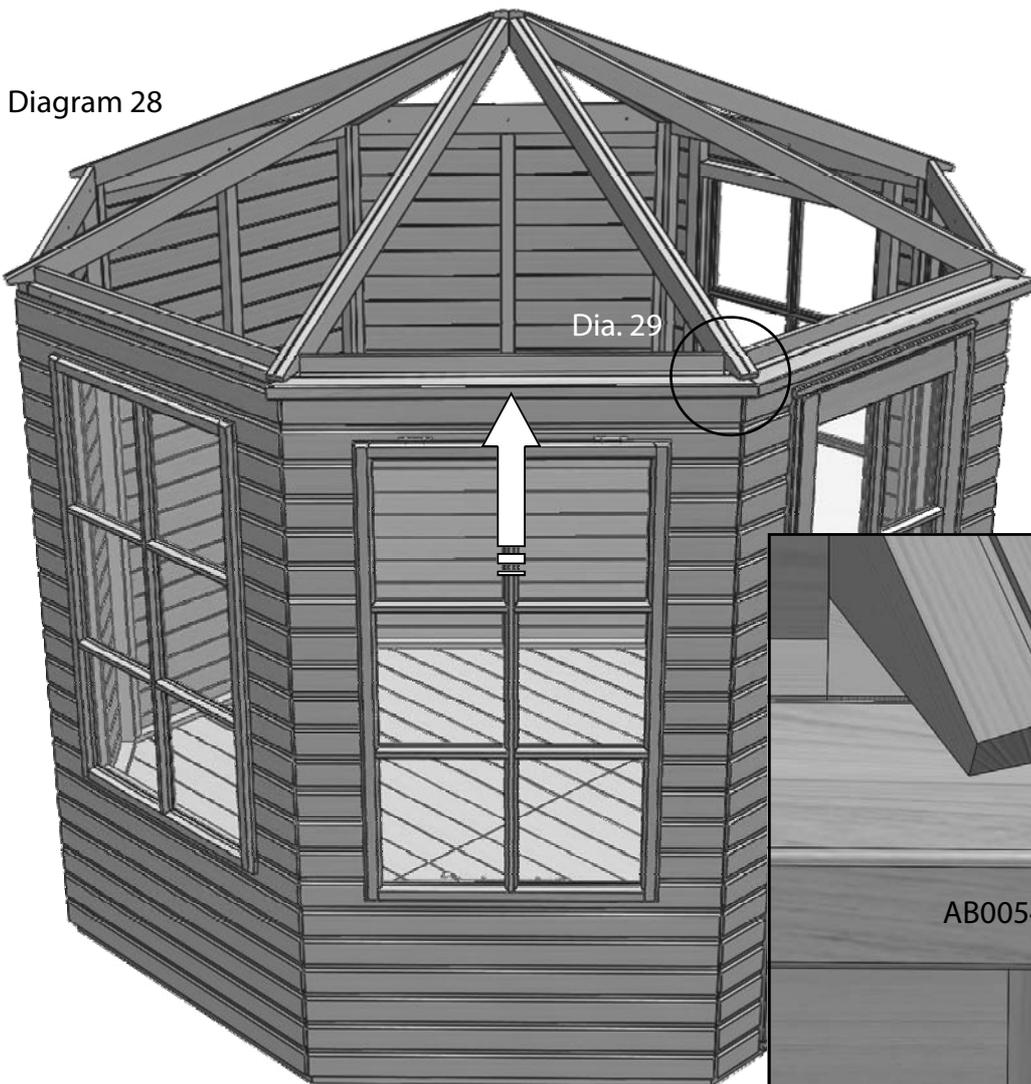
Work your way around the building making sure the ends of the soffits line up as closely as possible with the joint between side panels.
