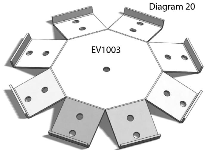
Working on the floor, slot the bracket onto the first roof bar. Drill pilot holes through the pre-drilled holes in the bracket. Then fix in place with 50mm countersunk stainless steel screws. Add another glazing bar in the opposite position to the last bar and fix this in place (diagram 21).
