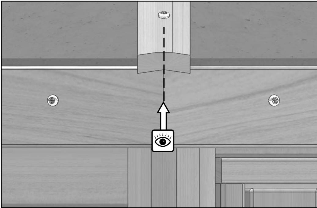
Once all the corner capping pieces are in position space the tops out evenly and fix into position.
