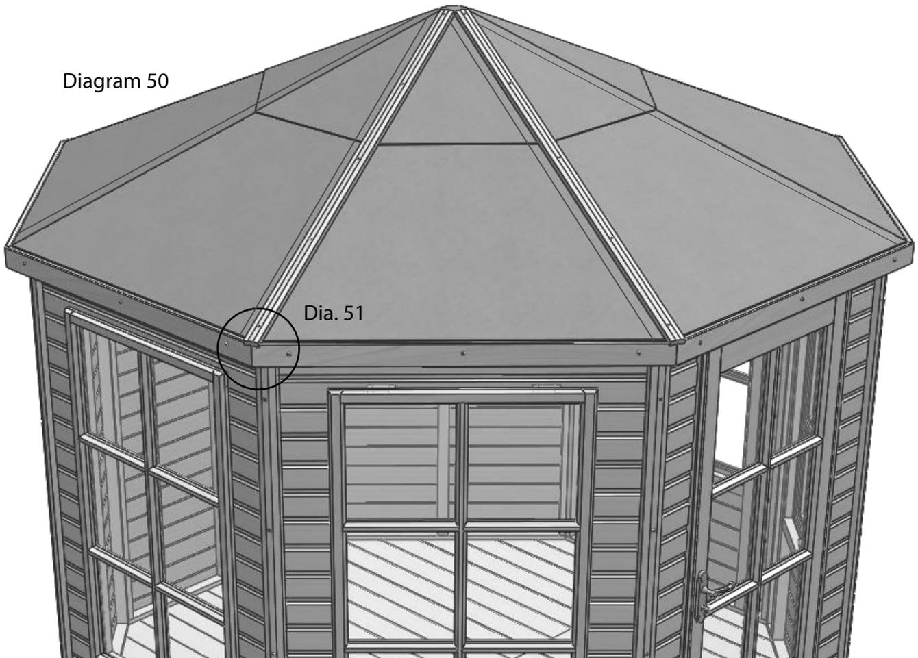
Now you can fit the capping working your way around the building. As you position each one, line the end up with the outer point of the joint between fascias (diagram 51). When you are happy fix in position with 50mm countersunk stainless steel screws. Only fix the bottom screw for now as you will want to fix the top screw next, when all have been spaced equally.
