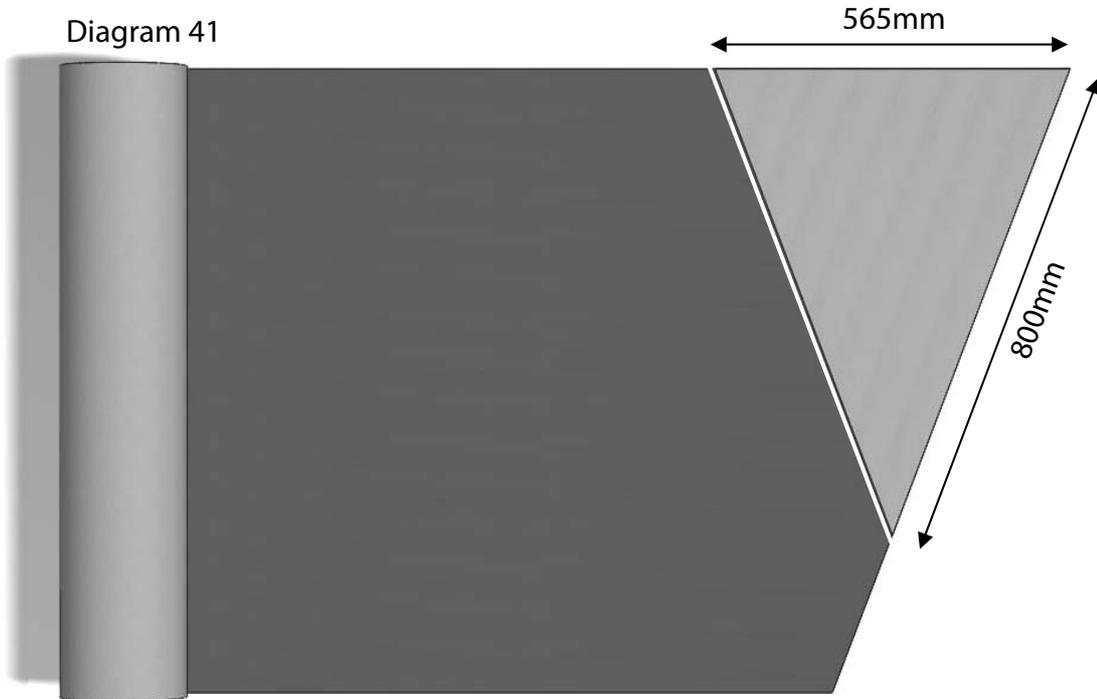
Lay the first large piece of roof felt onto the ply roof, this should have about 50mm overhang at the bottom of the roof. Using the clout nails provided fix the sheet to the roof. When nailing you should position the nail no more than 20mm from the joint in the ply sheets so the nail goes into the roof bar. The nails should also be no more than 300mm apart (diagram 42).
