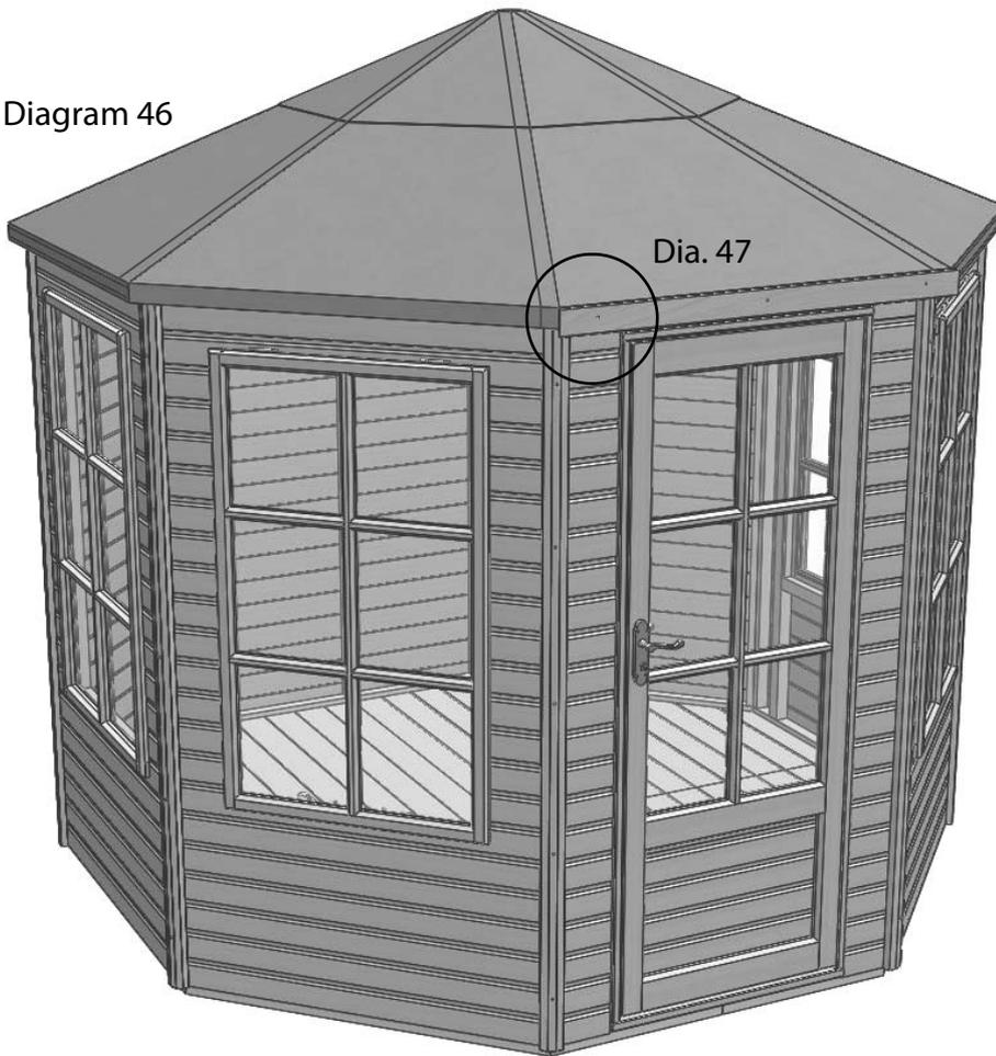
With all the felt in place you can begin to fix the fascias. Start with the fascia above the door. You will notice the holes are slightly off-set, in this install they should be closest to the top of the fascia.
