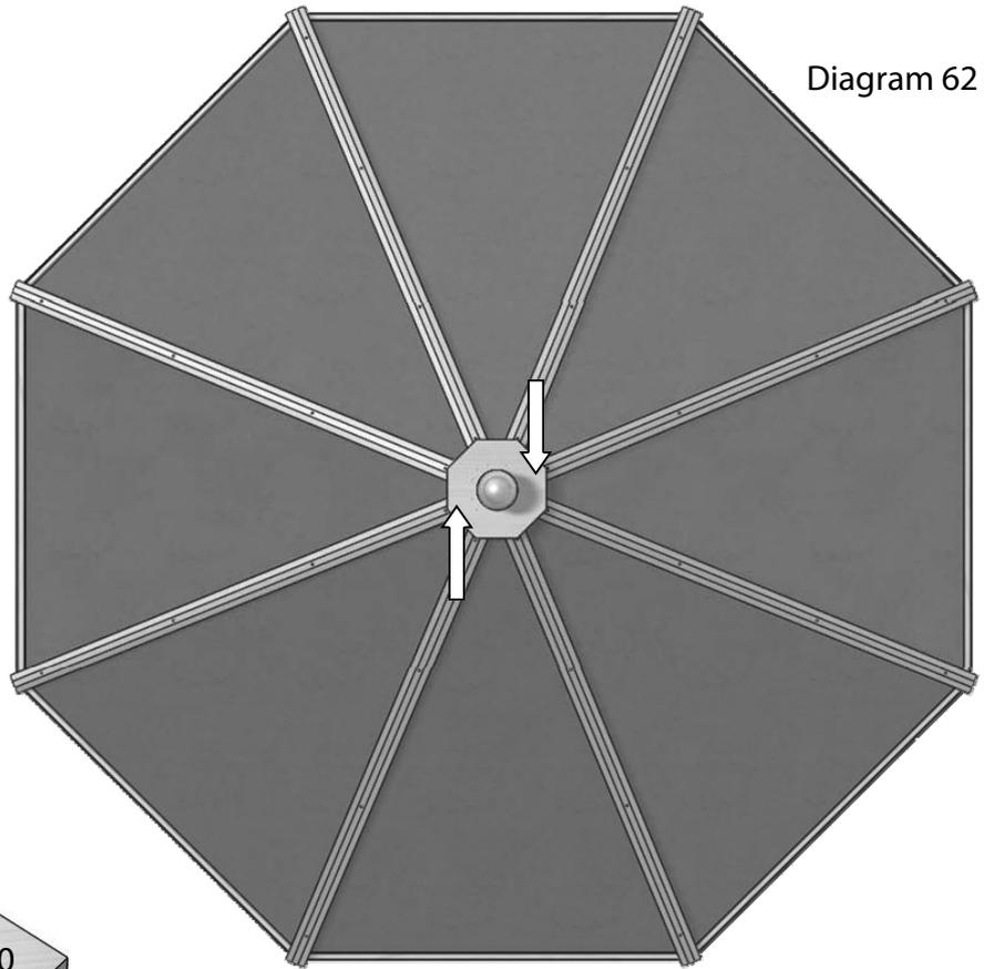
Line the corners of the top cap up with the roof capping, drill 2 or 3 pilot holes through the cap above the tops of the roof capping. Fix in place with 40mm pan head stainless steel screws (diagram 62 and 63).
