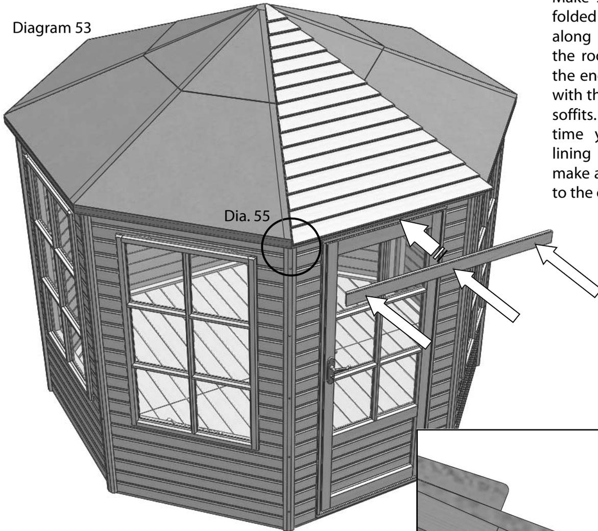
Make sure the felt is folded down tight along the bottom of the roof, also line up the ends of the fascia with the corner of the soffits. The more time you take over lining these up will make a big difference to the overall finish.
