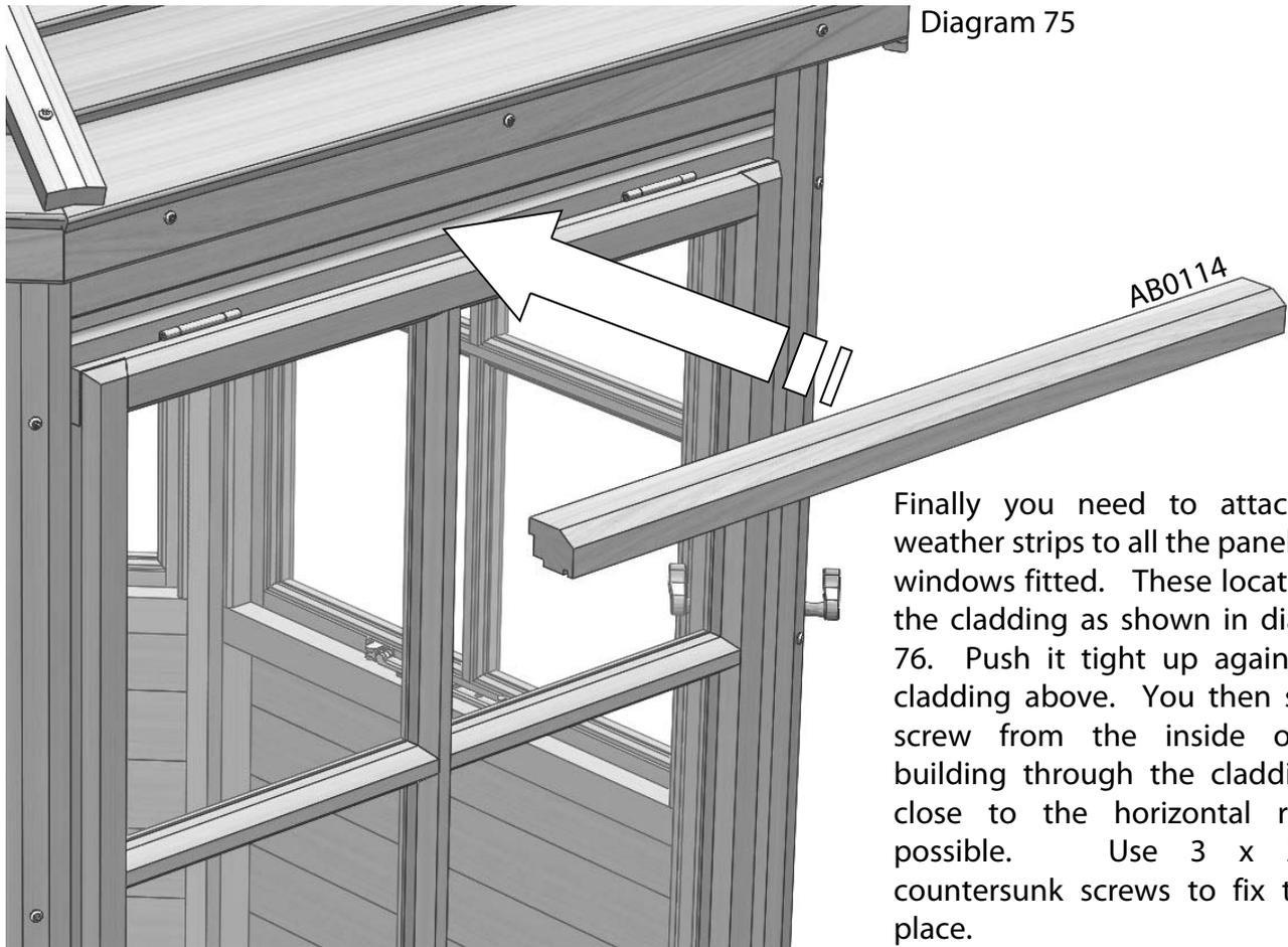
Finally you need to attach the weather strips to all the panels with windows fitted. These locate with the cladding as shown in diagram 76. Push it tight up against the cladding above. You then simply screw from the inside of the building through the cladding as close to the horizontal rail as possible. Use 3 x 25mm countersunk screws to fix this in place.
