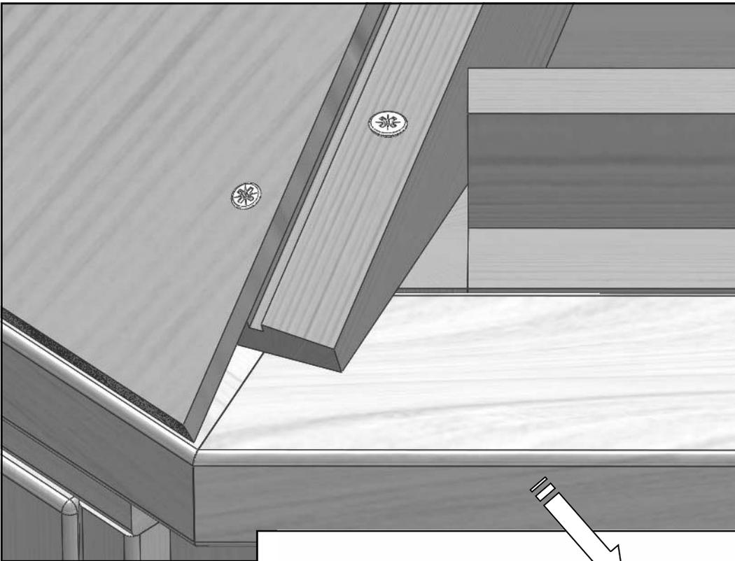
Make sure the ply roof sheet does NOT protrude past the soffits.
