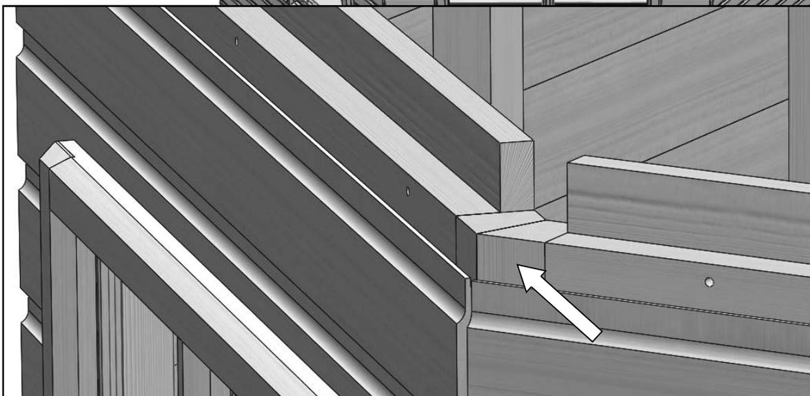
With all the side sections in place you can now install the door. Remember do **not** fix the sides to the floor yet.
