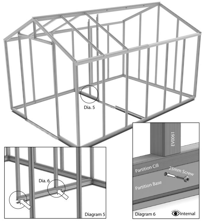
When in position, with the base flush with the end of the cill in the doorway (circled in diagram 5), fix with two 25mm screws at the two points shown in diagram 5. Keep this section supported until you fit the roof bar in the next step.
