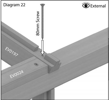
Fix the bottom of the partition roof glazing bars to the eaves bar with 80mm screws. Make sure the inside face of the glazing bar is flush with the eaves bar (shown below).
