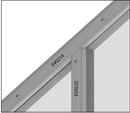
Once all the partition glass is in place you can finally secure it along the top edge with the roof bar capping.
