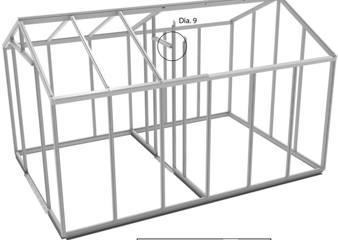
Next fit the opposite side to the aluminium base, again with two 25mm screws. With this section supported insert the door header into the mortise holes in the gable bars (diagram 9).
