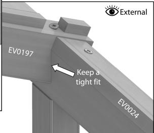
Once the bottom joint is fixed you can screw the glazing bar to the ridge (diagram 23). Do this with a 50mm screw but make sure the glazing bar is all the way into the joint. Diagram 24 shows an X-ray view of the end of the ridge. This shows the best angle for the screw. Again you want to be careful the end of the screw doesn't come through at any point.
