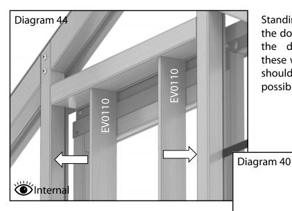
Standing on the inside of the greenhouse, with the door in the closed position you can install the door frame sides (diagram 43). Secure these with four 40mm screws per side. These should be fitted as close to the door as possible while still allowing it to pass by freely.
