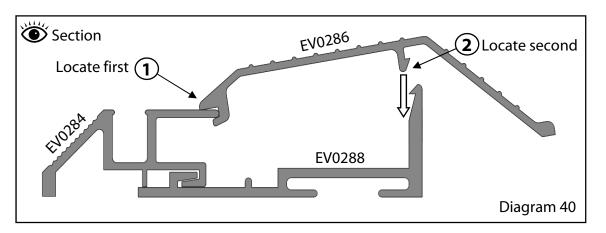
Next install the bottom door guide (EV0284) onto the door cill (EV0288) shown in diagram 40. Make sure the channels are free from grit and that this locates properly as you may find the next stage difficult if this is not the case.
