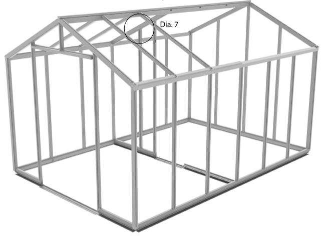
Slot the roof bar into position as you did before with the standard roof bars. Line up the gable bars with the slots in the roof bars and secure with 40mm screws. Don't secure this bar to the ridge or eaves bar at this stage as you will need some adjustment when fitting the partition side bar.
