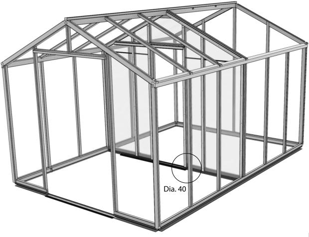
You can now fit the top door track to your partition. The right hand end of the door track should be roughly inline with the outer edge of the glazing bar below it (circled below). With help slide the door onto the track making sure the door wheels locate with the door track as shown in diagram 42, point 5. At the same time you need to locate the door guide with the door runner, point 6.
