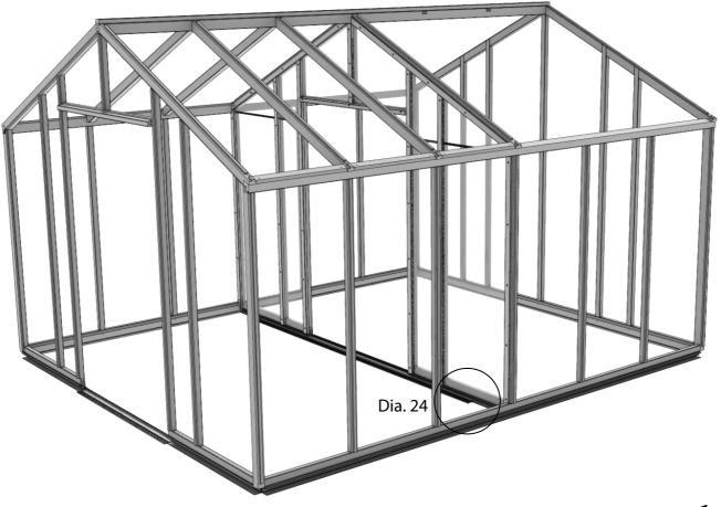
You can now fit the top door track to your partition. The right hand end of the door track should be roughly inline with the outer edge of the glazing bar below it (circled below). With help slide the door onto the track making sure the door wheels locate with the door track as shown in diagram 25, point 6. At the same time you need to locate the door guide with the door runner, point 7.
