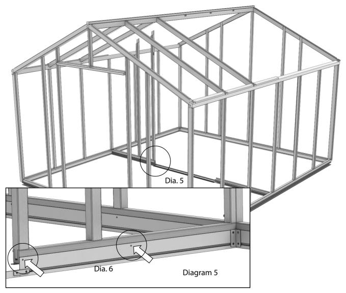
When in position, with the base flush with the end of the cill in the doorway (circled in diagram 5), fix with two 25mm screws at the two points shown in diagram 5. Keep this section supported until you fit the roof bar in the next step.
