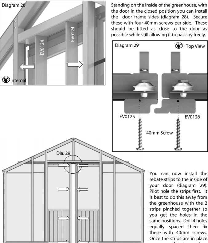
same positions. Drill 4 holes equally spaced then fix these with 40mm screws. Once the strips are in place you can fit the door handles on the inside, simply line these up with the handles on the outside of the door.
