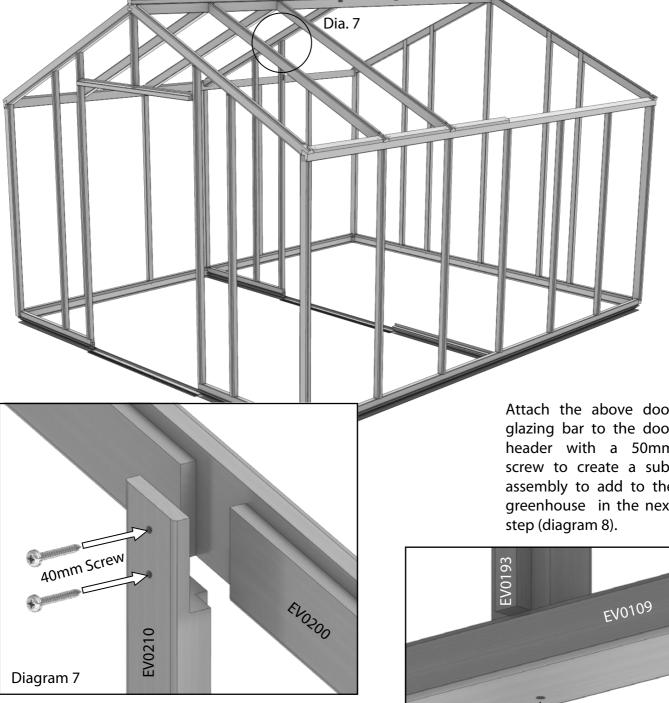
Slot the roof bar into position as you did before with the standard roof bars. Line up the gable bars with the slots in the roof bars and secure with 40mm screws. Don't secure this bar to the ridge or eaves bar at this stage as you will need some adjustment when fitting the partition side bar.
