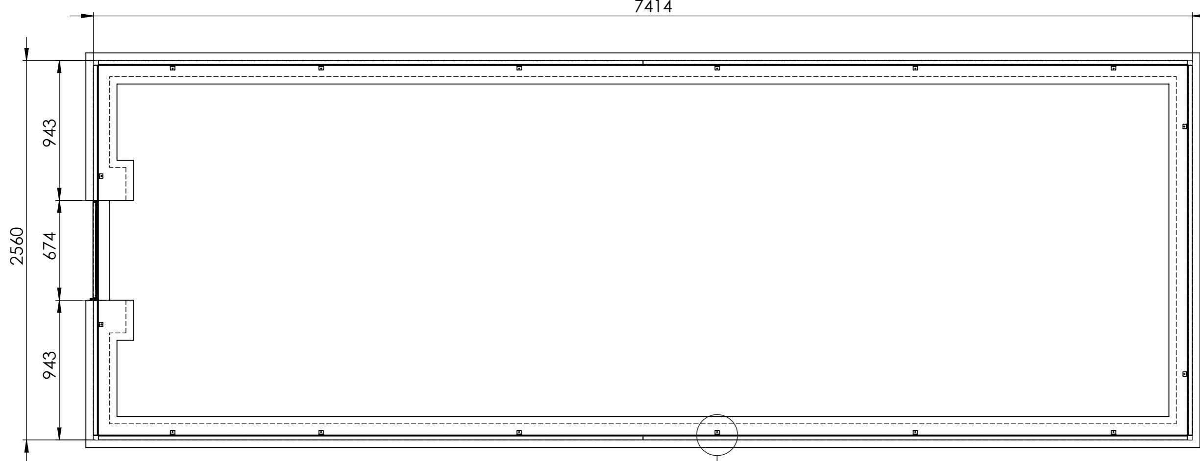
UK Please note: these dimensions are the outside dimensions of the framework and not the dimensions of the wall. You can determine the size of the wall depending on the brick and cover brick to be used.
