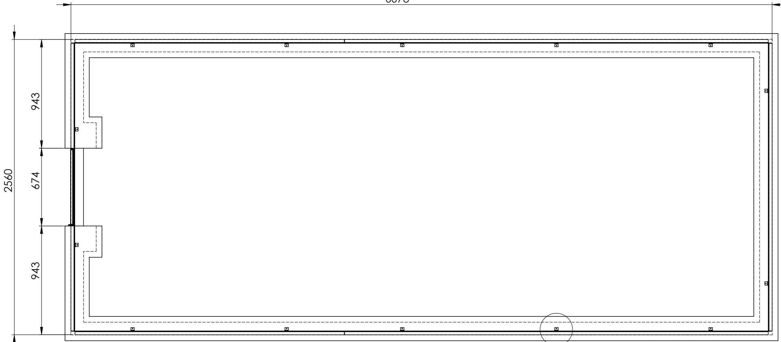
Please note: these dimensions are the outside dimensions of the framework and not the dimensions of the wall. You can determine the size of the wall depending on the brick and cover brick to be used.
