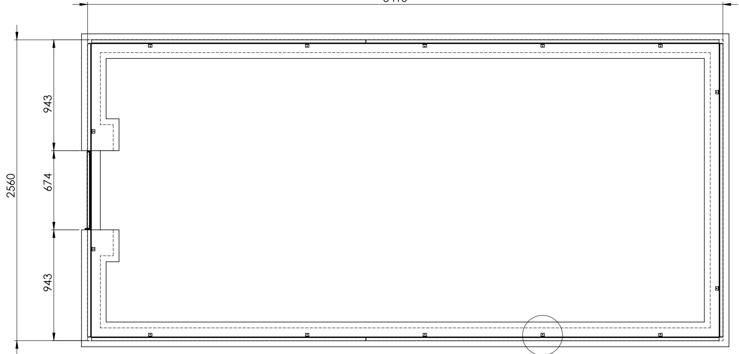
UK: Please note: these dimensions are the outside dimensions of the framework and not the dimensions of the wall. You can determine the size of the wall depending on the brick and cover brick to be used.
