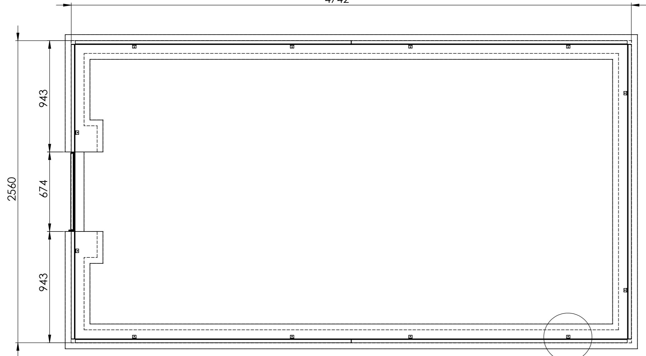
UK: Please note: these dimensions are the outside dimensions of the framework and not the dimensions of the wall. You can determine the size of the wall depending on the brick and cover brick to be used.
