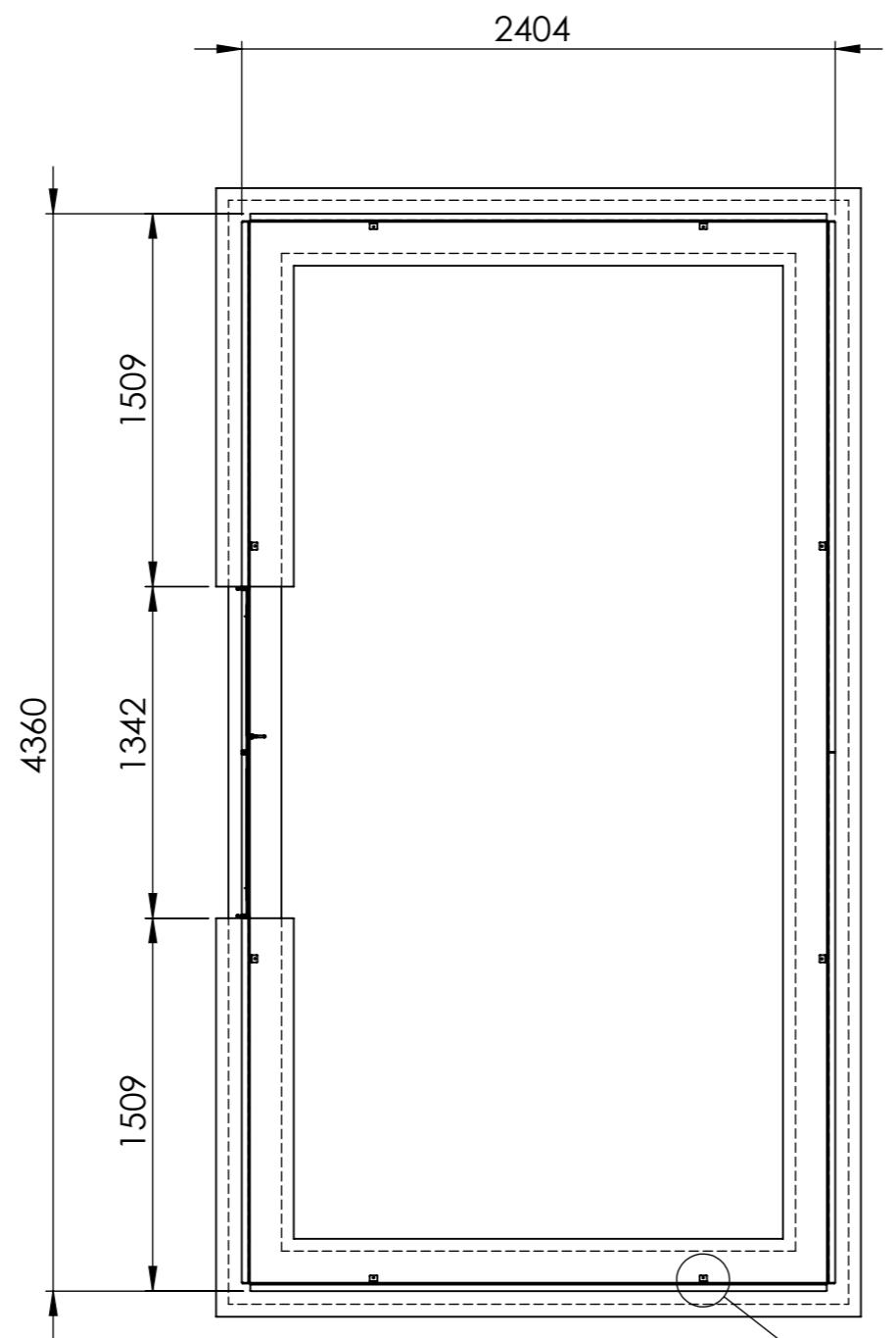
UK Please note: these dimensions are the outside dimensions of the framework and not the dimensions of the wall. You can determine the size of the wall depending on the brick and cover brick to be used.
